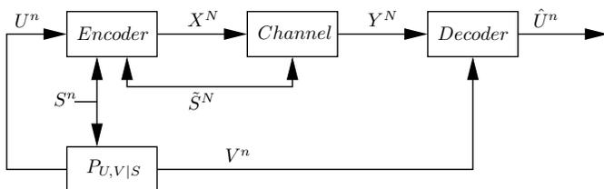
Fig. 2. Joint source-channel coding for the arbitrarily varying Wyner-Ziv source and Gel'fand-Pinsker channel, with side information at the encoder.
