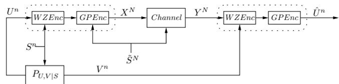
Fig. 4. An optimal separated scheme of a joint source-channel coding for the arbitrarily varying Wyner-Ziv source and Gel'fand-Pinsker channel, with side information at the encoder.
